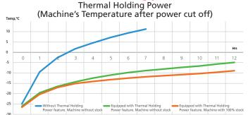
lce cream temperature would be 2°c to 5°c lower than machine temperature. In the event of loss of electric power, this 12 hours thermal holding power feature, can protect ice cream from melt. This can reduce losses and ensure highest ice cream quality and customer satisfaction
