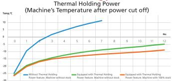
Ice cream temperature would be 2°c to 5°c lower than machine temperature. In the event of loss of electric power, this 12 hours thermal holding power feature, can protect ice cream from melt. This can reduce losses and ensure highest ice cream quality and customer satisfaction
